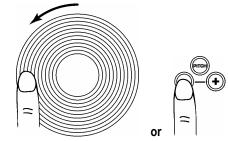
When Player 2 is ahead rotate the jog wheel counter-clockwise or press to bend pitch slower.
